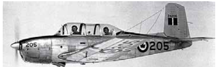
Mentor 24205 in regular RCAF service, carrying the trainer scheme of the day. The fin, rudder, tailplanes, elevators, wing tip caps and ailerons were 1-GP-12b Yellow 5-2.
