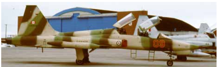
An early photo CF-5D 116809 in its Lizard scheme. Note the lack of 419 Sqn tail band and the lack of 'slime' formation light strips. (Robert Bryden photo)
