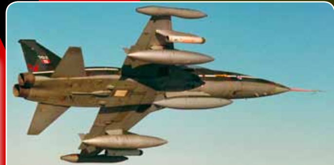
1981 - 702 . Under both wings are LAU-10 ZUNI rocket pods. Note the mix of colours on the pylons and fuel tanks. DND Canada photo AEC 81-327
