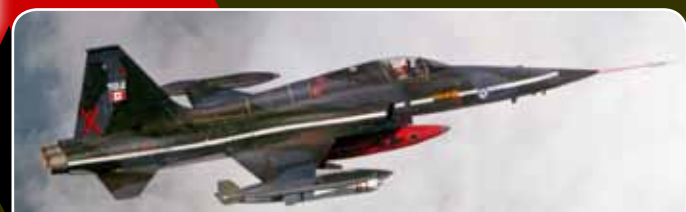
1986 - 702 with the flight test nose, carrying AETE's custom-built centreline camera pod. Just visible on the starboard wing is Mk. 20 Rockeye CBU. DND Canada photo AEC 86-787
