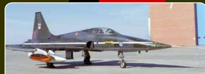
1981 - 702 with the flight test nose pitot, carrying a flight test orange camera pod. Note the silver-painted pylons and, unusually, a single fuel tank under the wings. DND Canada photo AEC 81-416
