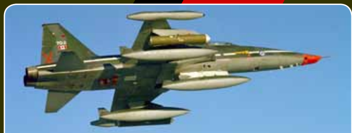
1978 - 702 sporting an orange-painted modified CF-5A/R recce nose. Under the wings are LAU-5002 rocket pods. Cameras are installed where the arresting hook normally resides. DND Canada photo AEC 78-13
