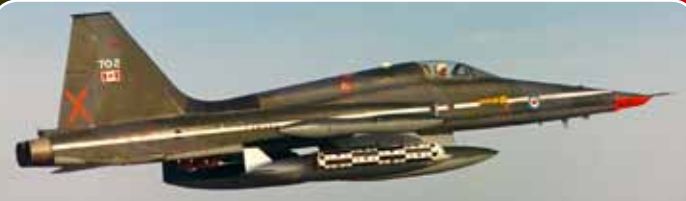
1976 - 702 sporting a CF-5A/R recce nose painted in flight test orange. Under the starboard wing is a four-shot LAU-10 ZUNI rocket pod and a silver-painted CF-5 fuel tank. DND Canada photo AEC 76-53
