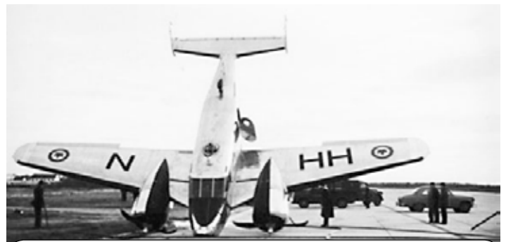
An RCAF Expeditor in an undignified pose, but nicely showing off the code letter placement, anti-glare and leading edge de-icer boots. (RCAF photo)
