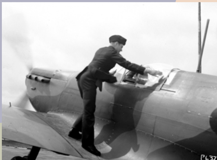
Another good close-up that nicely contrasts the generally good condition of the paint job against but the moderate booting scuffing seen at the wing root paint. The unpainted wing fillet fasteners are also evident. Is this last feature perhaps the result of the aircraft being crated and shipped to the USA, from where it was re-shipped and finally re-assembled in Canada. DND Canada photo PL-377, 16 May 1940
