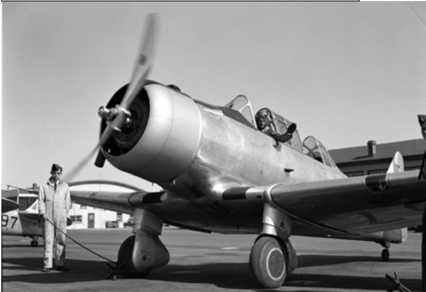
A Yale very early in service at RCAF Stn Borden before the exhaust stack was extended and the wheel pants were removed. DND Canada photo PL-2222
