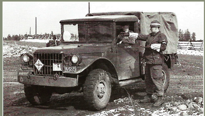
▲ An M37 3/4 ton truck in Alberta in 1968. Mounting the FMC decal on sheet metal and then attaching it to the grille was a typical solution to display the marking and better protect it compared to applying it to the bumper. (DND Canada photo IE68-50a)
