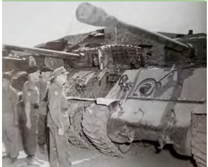
▼ Inspection of the Canadian Brigade Commander, Lt-Col. Jean Allard, of LdSH A Sqn's tanks in September 1953. You can see the moved machine gun mount on the turret top, and the Centurion tank tracks added to the turret sides. The tank on the right is a replacement vehicle brought into service, lacking the extra stowage. The hull machine gun is also missing in the "ball" mount. (Library and Archives Canada, DND photo via Anthony Sowards)
