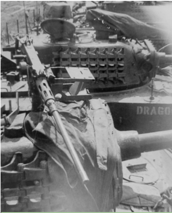
▲ A tank of D Sqn in August 1954, Royal Canadian Dragoons (which was a mixed squadron with members of the Armoured reserve). The photo shows the relocation of the turret machine gun on the turret top and the added Centurion tank tracks. Also note the extra radio antenna on the Sherman tank next to the one in the photo, suggest that this one might be a command vehicle, which had an extra radio to talk to other units. (Royal Canadian Dragoons Archives via Anthony Sowards)
