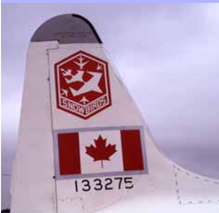
▼ Tail detail of '275. The small black bars are alignment indicators showing the 'locked' position of the panel fasteners
