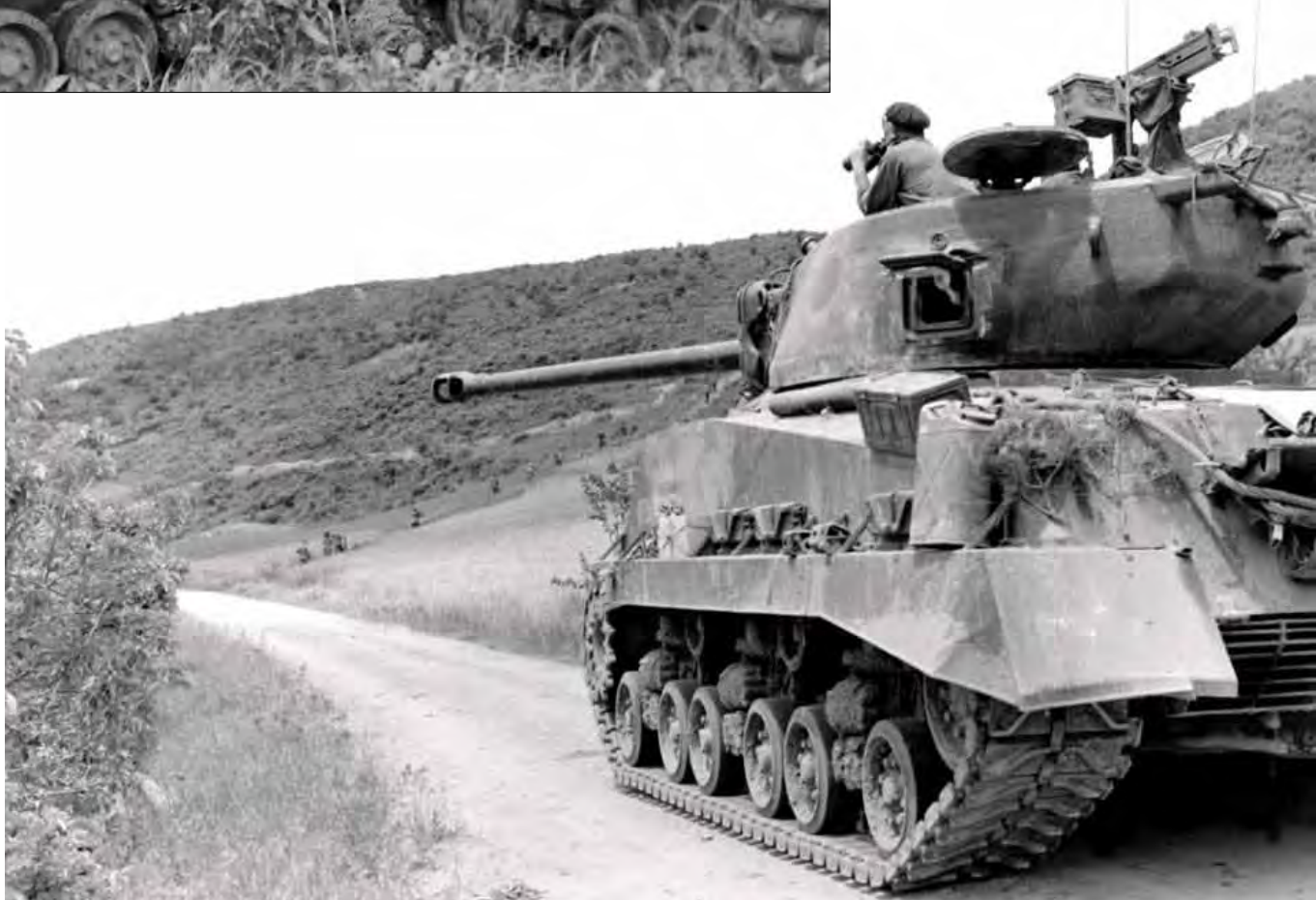
▼ A tank from the Strathcona's C Sqn's 3rd troop named "CATAWABA" provides overwatch security for members of 2nd Battalion of the Royal Canadian Regiment. The tank still retains part of the sandshields on the hull sides. The crew has added extra stowage to the hull sides and an extra water jerry can has been mounted on the rear. (Library and Archives Canada, DND photo via Anthony Sowards)
