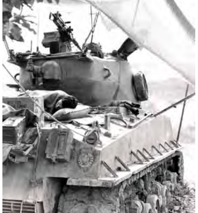
▼ A C Sqn tank in a defensive position along the Imjin river in September 1951. A great photo that shows typical crew stowage; the square box mounted on the back plate is the tank telephone, used by the infantry to talk to the tank crew. The 25th Cdn Inf Bde marking is seen on the rear plate. (Library and Archives Canada, DND photo via Anthony Sowards)
