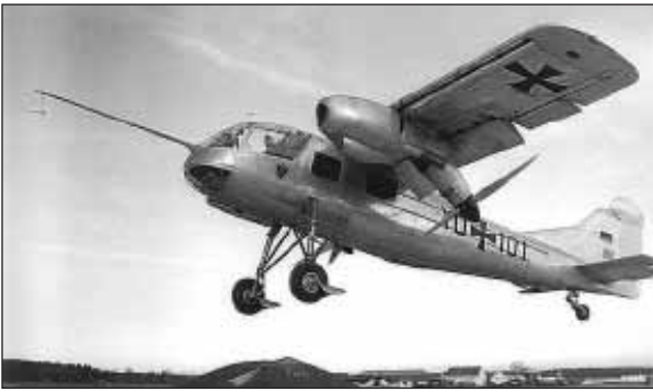
The Dornier Do-29 had pusher propellers that could droop down, for increased STOL capability. A resin kit is available in 1/72 scale from Unicraft.
