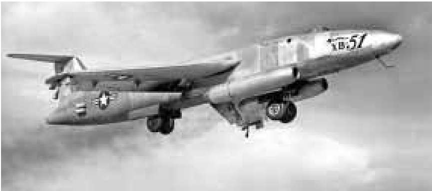
The Martin XB-51. In addition to the two engines hanging from the fuselage, there's another one in the tail. I wonder if you could land on snow with the wheels up! Beaver Corporation (no, it's not Canadian – it's Japanese) has a 1/72 version.
