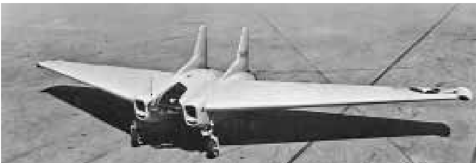
The XP-79 “Flying Ram” (!) It's a lot smaller than it looks, with the pilot lying prone in the nose. I seriously doubt he would want to “ram” anything in that configuration. RS Models has a 1/72 version.
