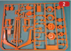
(Fig. 2). There are prominent mould lines on every part and quite a few sink marks. Fortunately most of the ejector pin marks visible are raised and easy to take care of. The instructions
