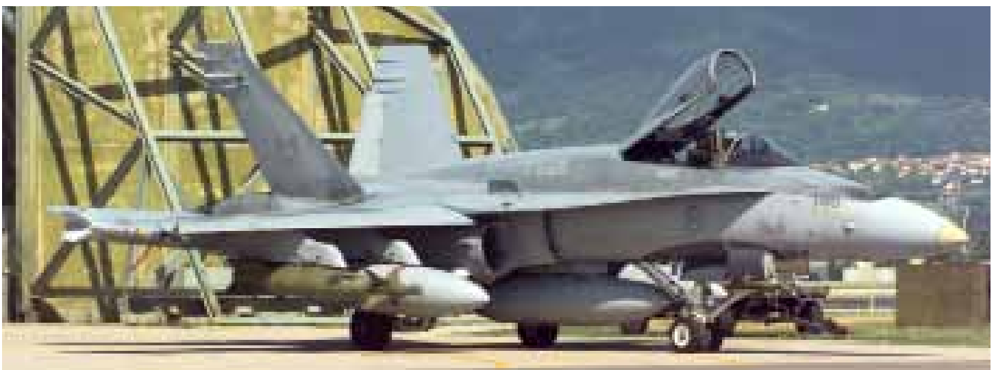
188746 loaded with two GBU-10s, AIM-9Ms and an AIM-7M. Note the evident wear and tear on the Mk. 84 bomb body. DND Canada photo CKD99-2094-06
