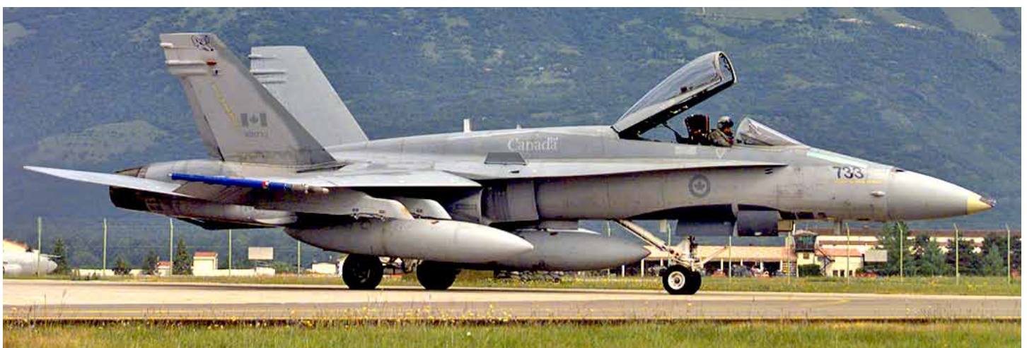
188733 taxiing during a training mission. It is carrying a CATM training missile in place of an AIM-9M. Note the damage repair on the front of the radome and the replaced AAR probe door. Two IFR probe damage stencils are applied just under the LEX. DND Canada photo CKD99-2120-04
