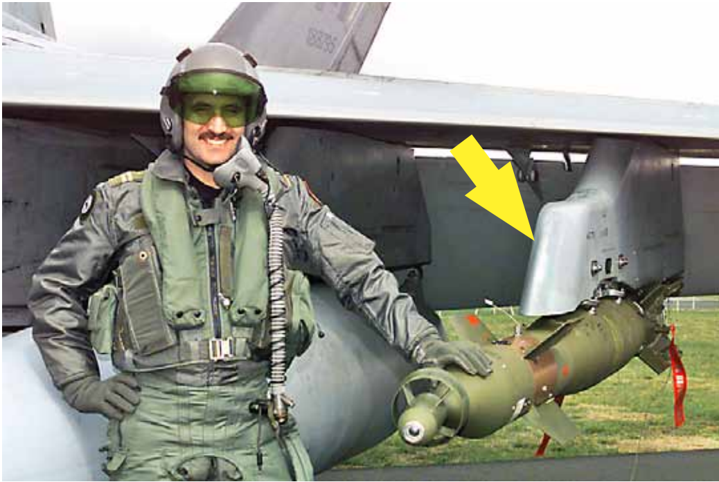
A CF-18 pilot in the US-style flight gear worn for this deployment. His hand is resting upon a GBU-12 500-lb LGB. The SUU-63/A pylon is the standard 'skinny' type, with just a plain metal leading edge. DND Canada photo CKD99-2017-02
