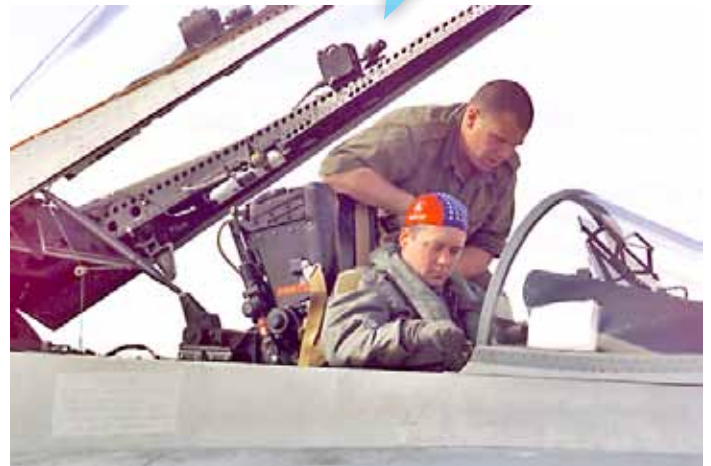
This view of a CF-18 pilot strapping in for a flight shows some great cockpit and canopy detail. Note the two video cameras mounted on the canopy frame. DND Canada photo CKD99-2067-05
