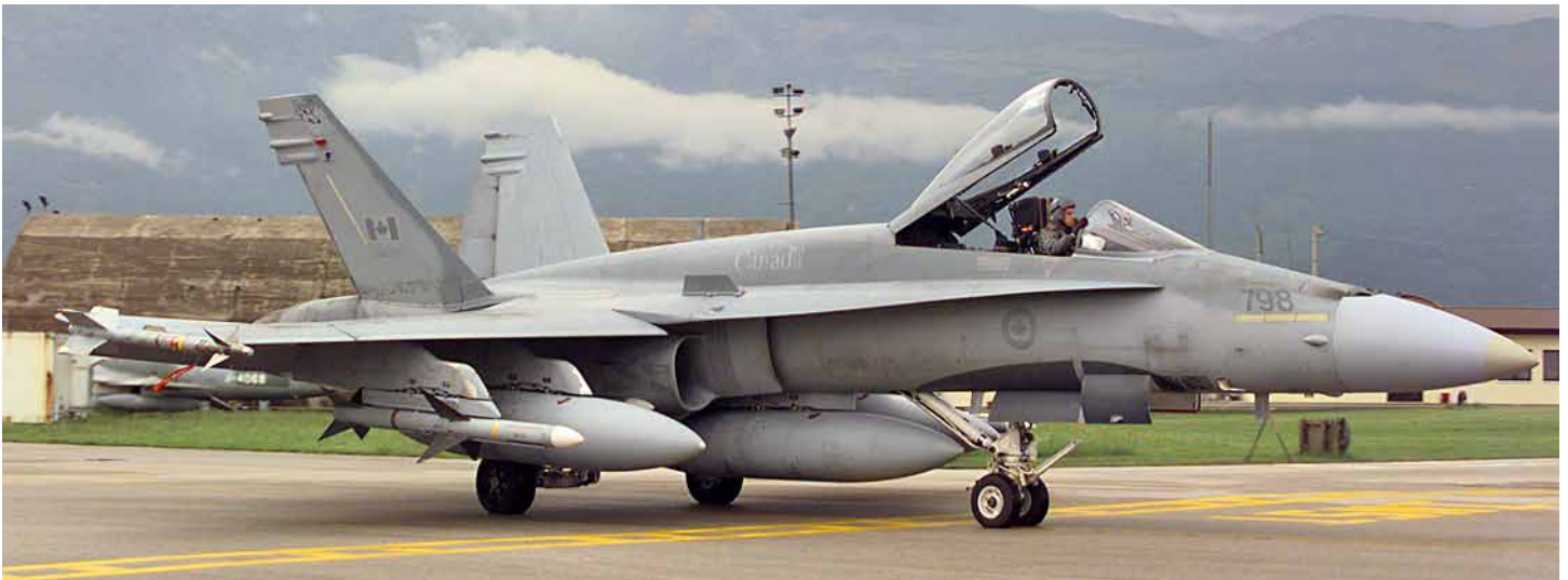
188798 loaded for an air-to-air mission. AIM-9Ms and AIM-7Ms are the only weapons visible. This was earlier in the Roto 3 deployment, as the RT article showed that 798 later had two IFR probe damage markers under the LEX. Note the camouflage demarcation dips down from the LEX to the night formation light. DND Canada photo CKD99-2066-05
