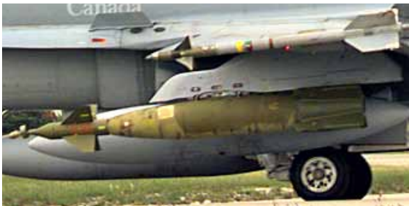
188753 taxiing for a mission. The night identification light has been removed and the window cover added. The Mk. 84 bomb body shows more weathering than the GBU-10 guidance kit (below). DND Canada photo CKD99-2041-08
