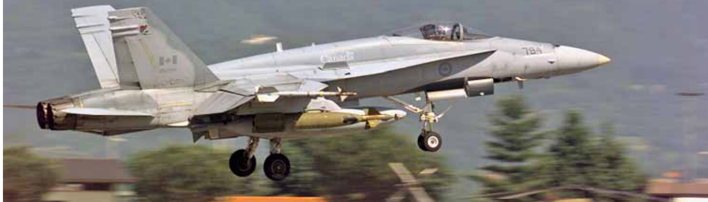
CF-18 188794 launching for a mission. Aside from the AIM-9M and AIM-7M, a GBU-10 is mounted on a 'fat' SUU-63/A wing pylon. DND Canada photo CKD99-2085-09
