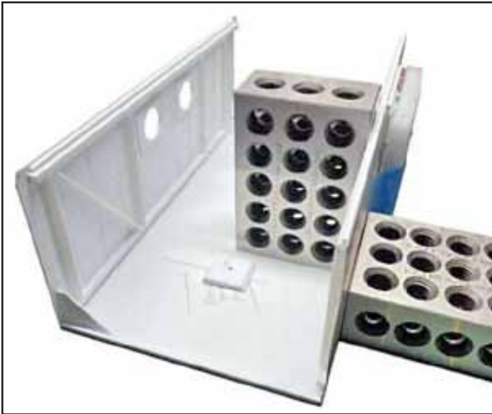
Squaring up the vehicle sides using 1-2-3 blocks.
