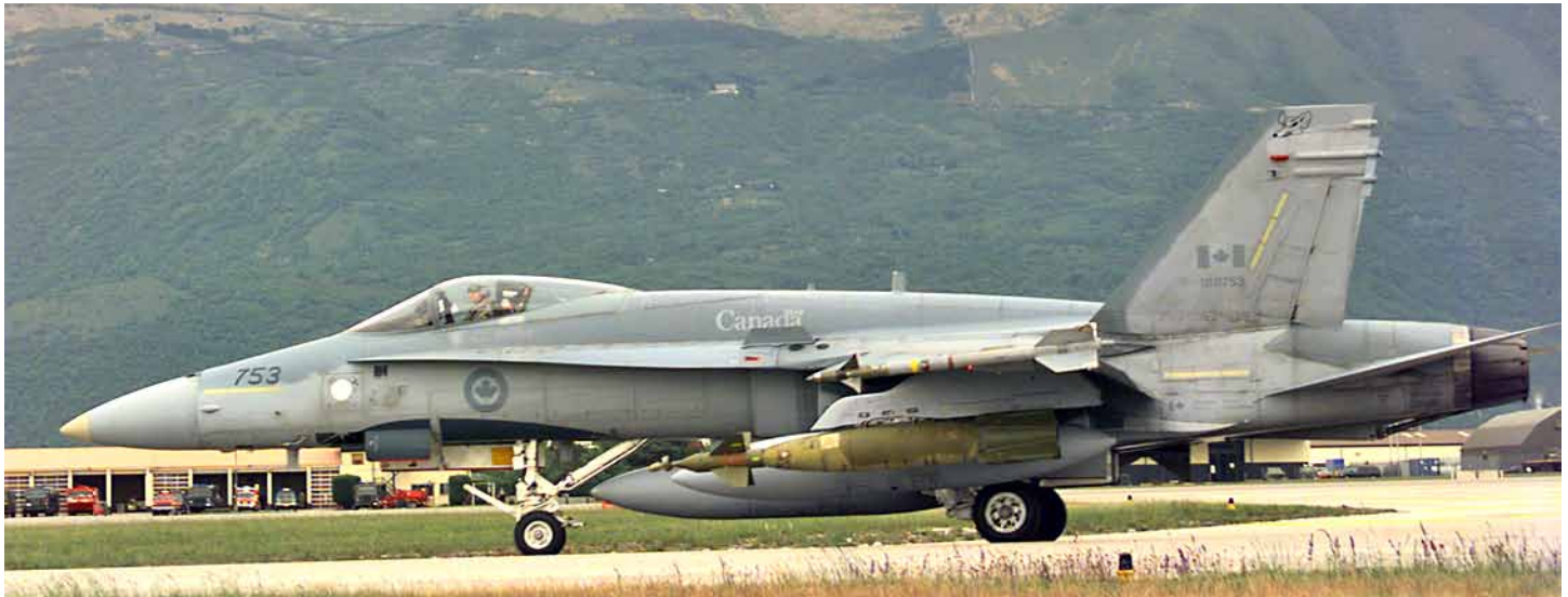
188753 taxiing for a mission. The night identification light has been removed and the window cover added. The Mk. 84 bomb body shows more weathering than the GBU-10 guidance kit (below). DND Canada photo CKD99-2041-08
