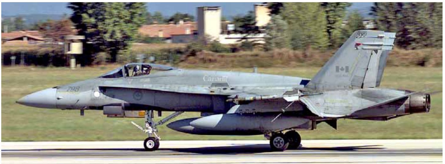
188798 armed with an AIM-7M and AIM-9Ms, presumably returning from a mission. Note the empty left outboard SUU-63/A wing pylon, which may indicate that a weapon was used. DND Canada photo CKD99-2145-03
