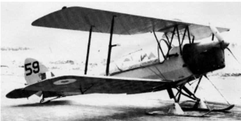
Fig. 10. Late wartime RCAF Tiger Moth RCAF serial number 9859, with the 'last two' numbers of the serial painted on the rudder. Again, note the early wartime-style fin flash and the 'Type A' roundel on the underside of the lower starboard wing. Credit: RCAF BE 450.
