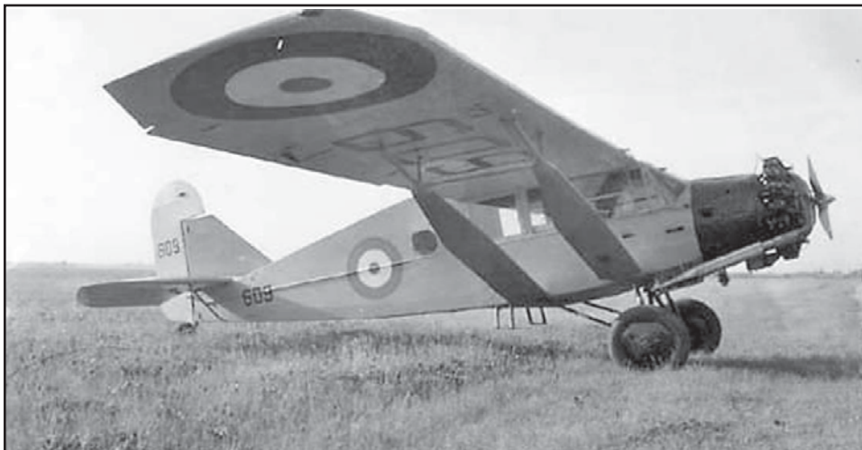
RCAF Pacemaker 609 on its wheeled undercarriage. These machines were reportedly finished overall yellow with black engine cowlings. This provides a good view of the broad airfoil struts.
