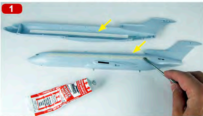
1 It is not enough to simply put putty in the window openings. A solid backing needs to be added, lest the putty just fall into the model, thereby accomplishing nothing.
