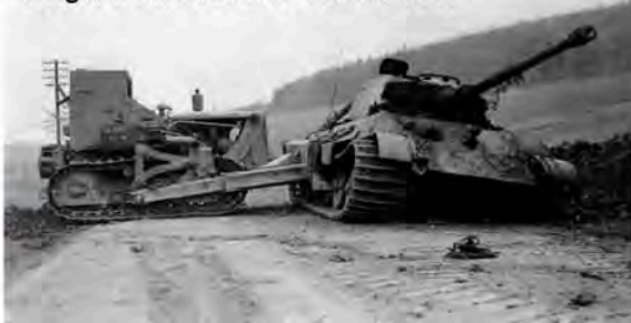
a D7 Armoured bulldozer pushing a Tiger II off a route in France 1944
