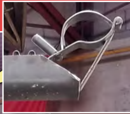
Rear view of turret showing lift rings, MG mount and L-channel brackets. Steve Sauvé photo, July 2018
