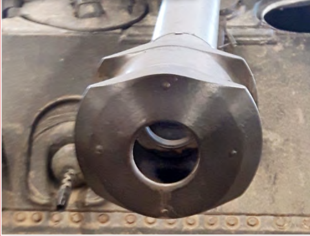
The business end of the Canadian M4A2's 76 mm gun. Sam Richardson photo, 2018
