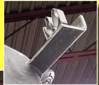
Right side of the turret rear. The L-channel on this side is square-cut. Note the shape of the open-bottomed fitting where the MG mount is located. Steve Sauvé photo, July 2018
