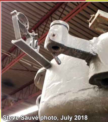
Left side of the turret rear. The L-channel on this side is angle-cut. Note the shape of the open-bottomed fitting where the MG mount is located. Steve Sauvé photo, July 2018
