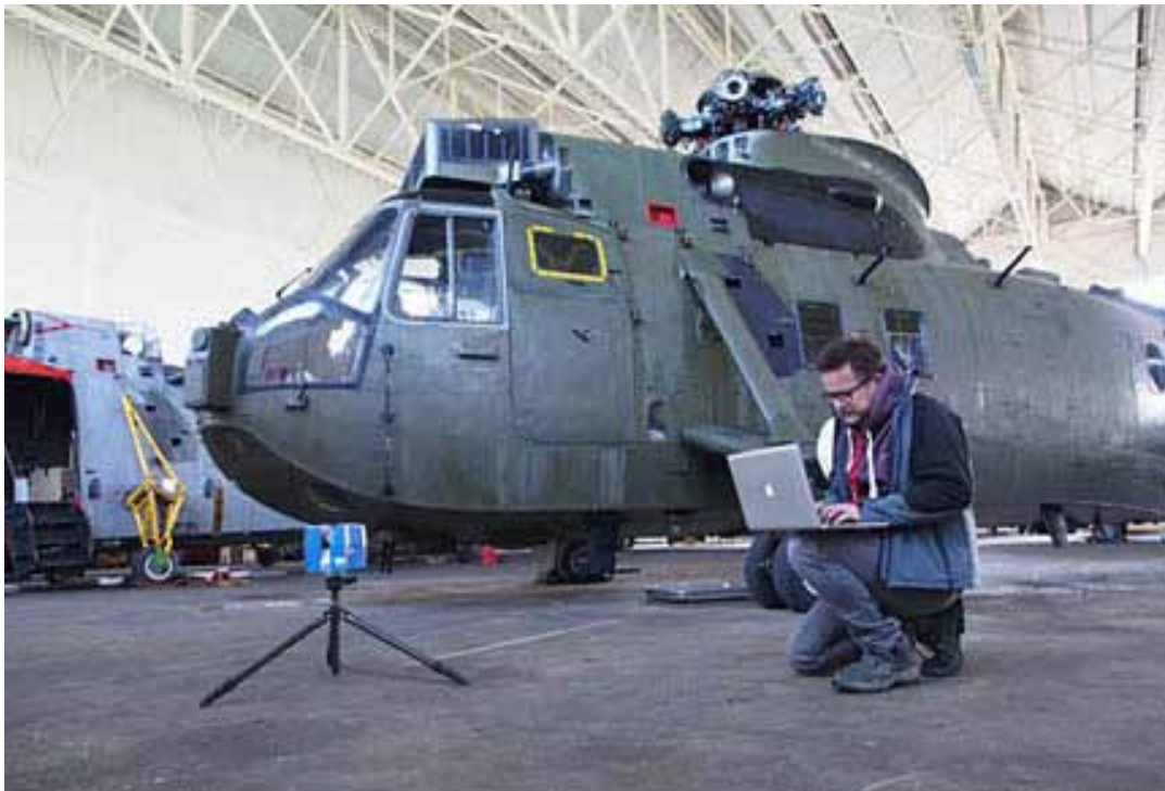
The Airfix LIDAE crew setting up the scanners around the Sea King.
