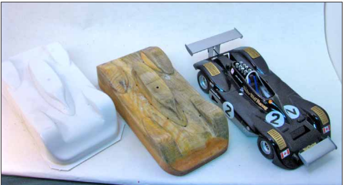
1:24 scale test body, wooden buck and finished model of Wolf Dallara
