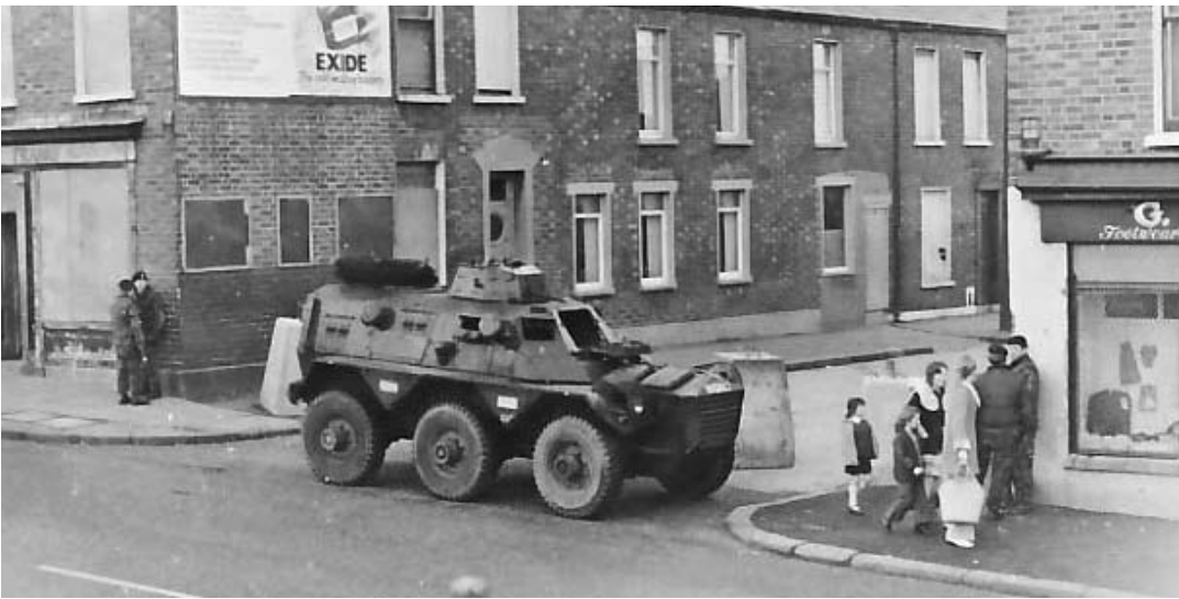
Saracen at a corner on the Crumlin Road, on the edge of the Ardoyne district in January 1973. Note the barbed wire coiled around the rear machinegun ring on the upper deck. Reflective tape has been applied to the mudguards between the wheels. The vehicle is No. 98-BA-52.
