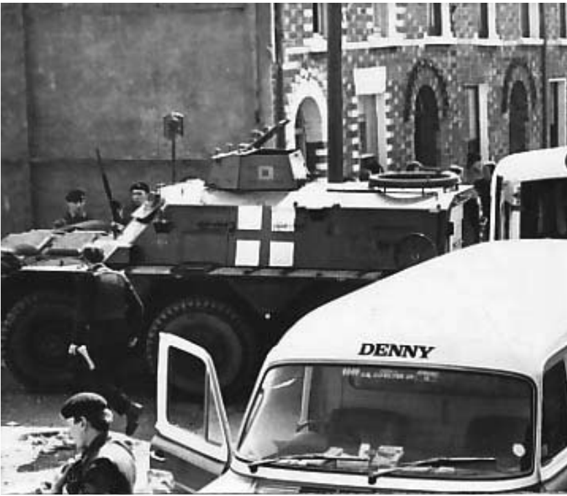
A Saracen ambulance attends an incident. The van in the foreground contained the body of a murdered Loyalist official, found August 23, 1972. Note the absence of a turret machinegun, and the mesh-enclosed beacon ahead of the turret. Also note the rather crude hand-painted red cross and the unusual square marking on the side of the turret.
