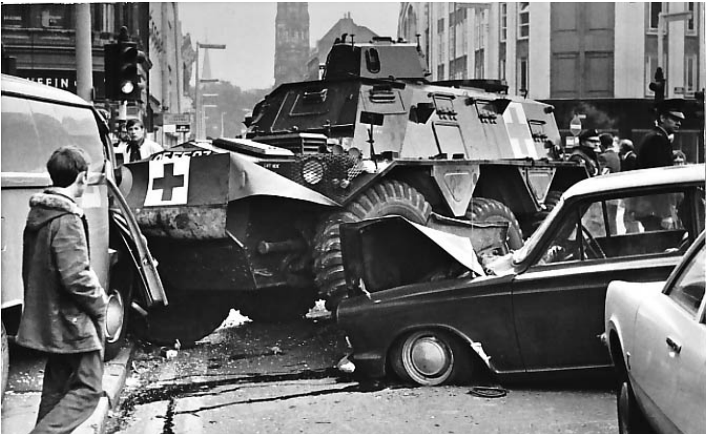
Aftermath of an accident, July 31, 1972. This Saracen ambulance No. 05-FF-07, an FV.603C, ran a red light on busy Royal Avenue in downtown Belfast, hitting several vehicles and injuring three people. Note the absence of a turret machinegun. The red crosses are neatly applied.
