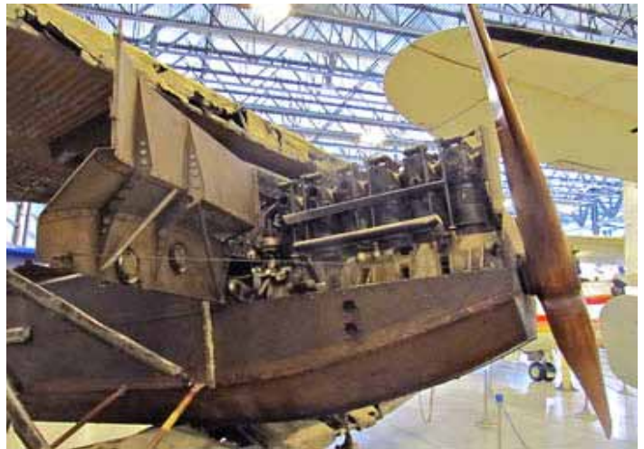
A close-up of the nose area. Note that the hinged engine cover panel has been swung open. You can get some idea of the thickness of the steel 'bathtub'.
