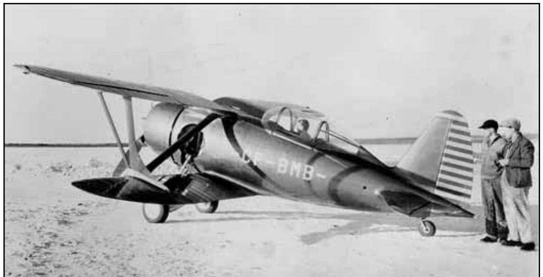
Pilot is in the cockpit preparing for flight. Were it not for the upper wing, the large canopy would have provided an excellent view all around.
