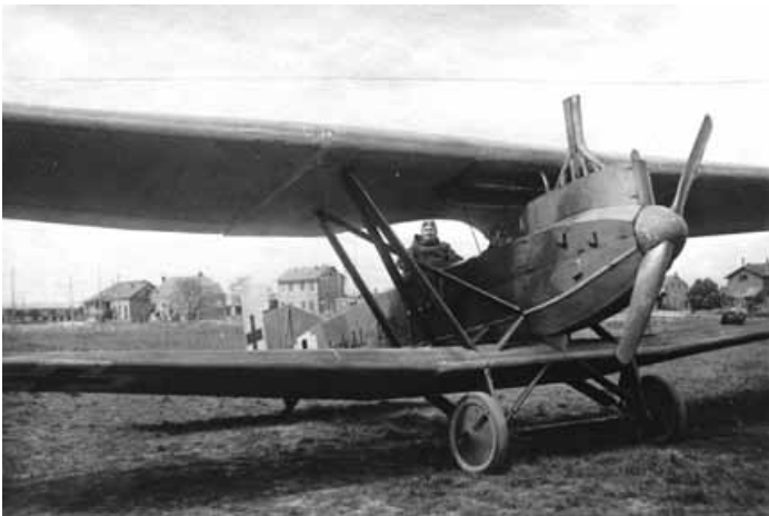
Another J.1 with the gunner standing up in his compartment. Note the prominent exhaust pipes.
