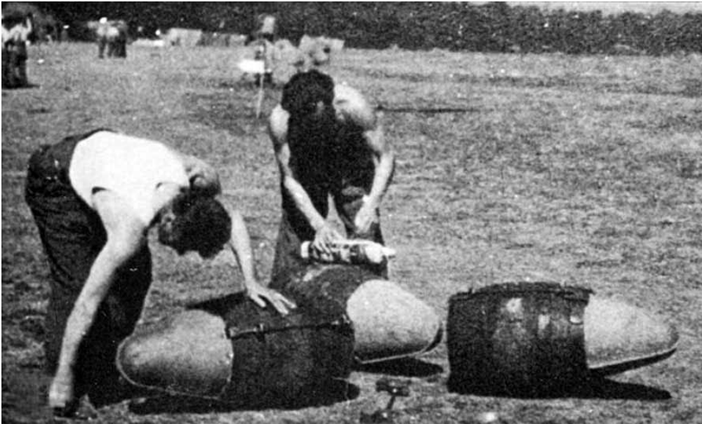
'Beer bombs', wooden kegs being fitted with streamlined 'nose cones' for transporting in bomb racks underneath Spitfires by members of 131 Fighter Wing, probably in August 1944 at Ford airfield in West Sussex.
