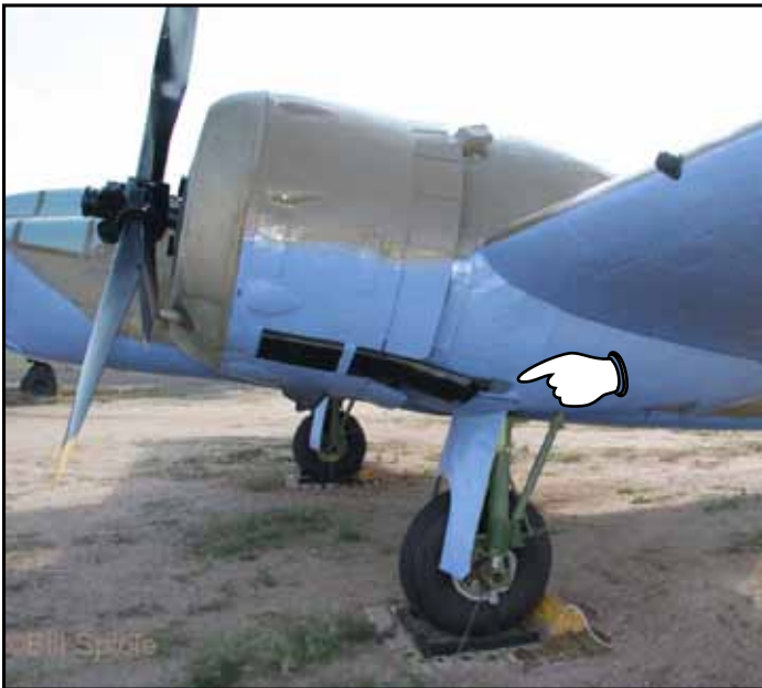
Cabin heater pipe at the rear of the exhaust.
