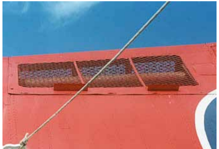
The large screen section on the upper fuselage is a cooling vent for the engine that is located below and slightly aft of it. Located inside the opening is the drive shaft that connects both rotor assemblies
