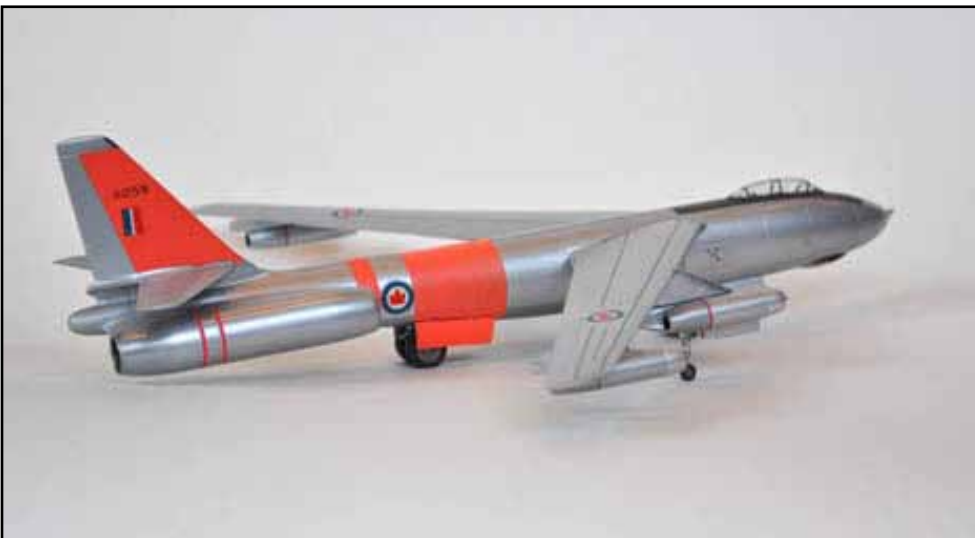
B-47 testbed aircraft with the Orenda Iroquois engine mounted to the fuselage.
