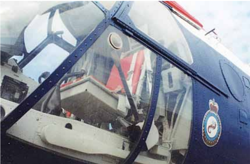
Details on the bulkhead include a couple of boxes with one supporting a large number of wires. This view shows that the first window on the port side has been either painted over or replaced with sheet aluminum. This is the location of the large oval escape hatch that was added later.
