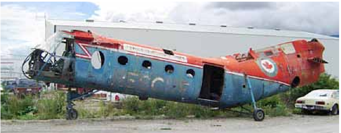
This airframe was photographed at Hope BC. Though a derelict, it shows well the location, size and configuration of the escape hatch that was added during service. Gary Fairfull Collection.
