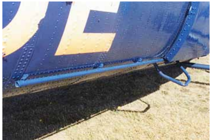
Close up view of the port door lower guide rails.
