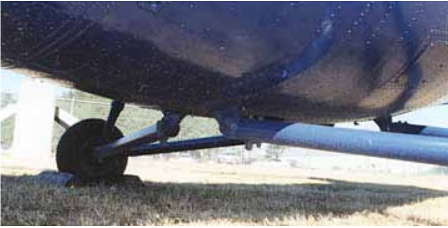
A view of how the main landing gear support struts are attached to the lower fuselage.
