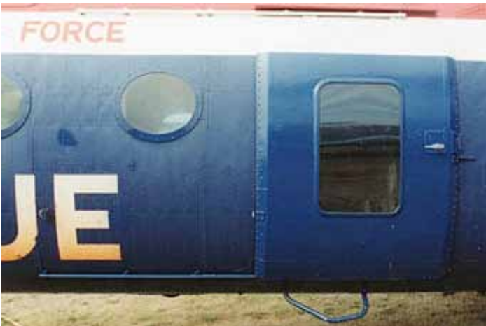
Main entry door that is located on the port side. Note the rail type guides both top and bottom.
