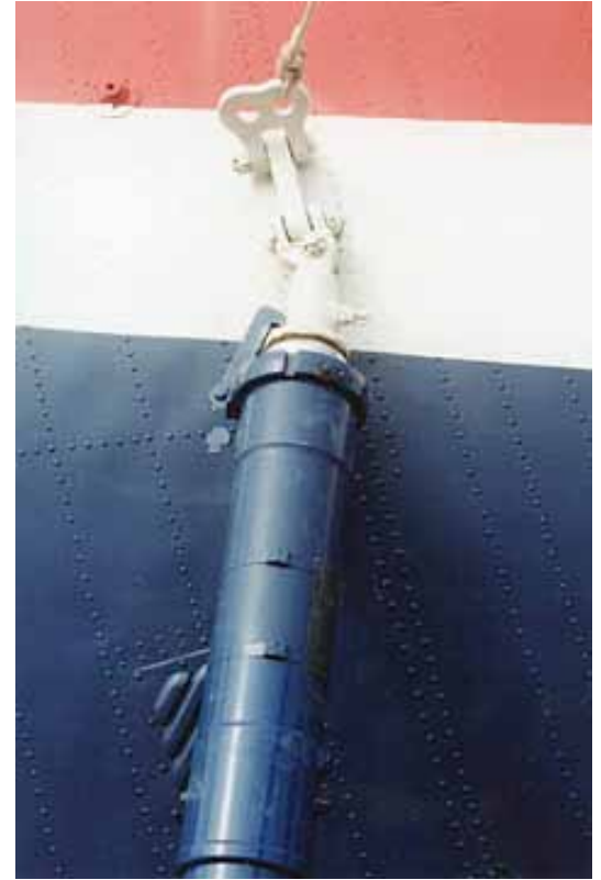
Close up view of the top of the port main gear strut clearly showing the double anchor station
