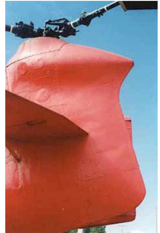
View of the end of the fuselage. This shows the two different sized access ports located below the horizontal tail.
