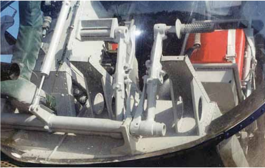
Note the two different types of foot pedal. Both are accurate, though perhaps not at the same time! Note the foot rest extension below the pedals and the green duct work on the center console.
