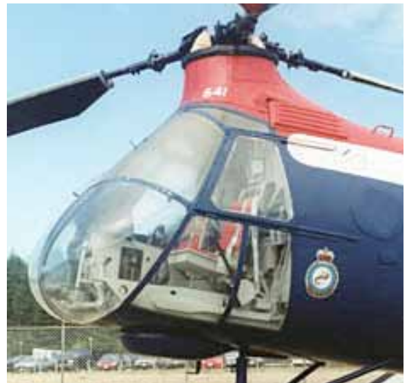
Port side of the cockpit, showing the raised framing that holds the aft-sliding side windows.
