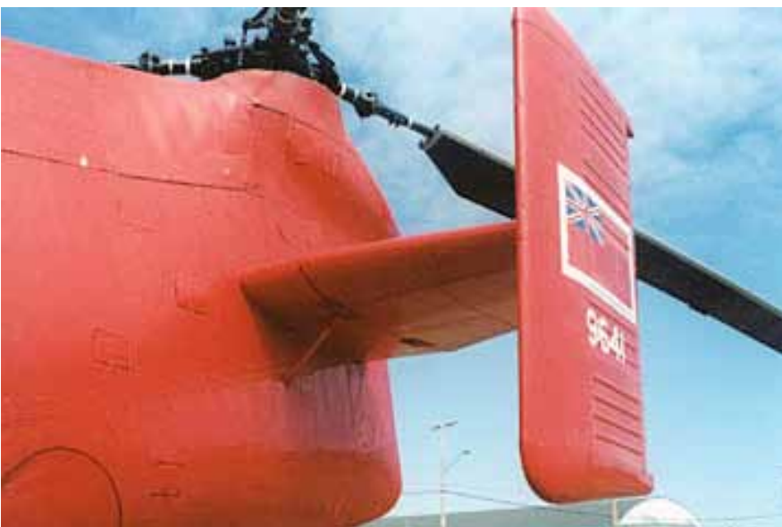
General view of the prominent tail of the H-21. Note the round access ports (missing from the Italeri kit) and the small support strut.
