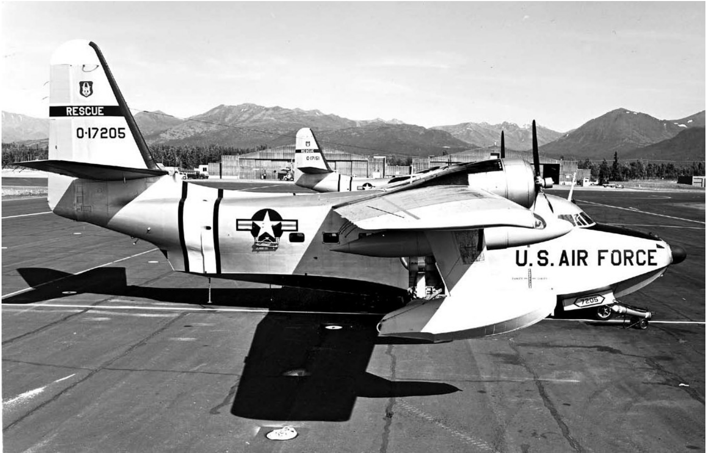
A USAF HU-16B. This camera angle makes it easy to see the leading edge camber on the wing
