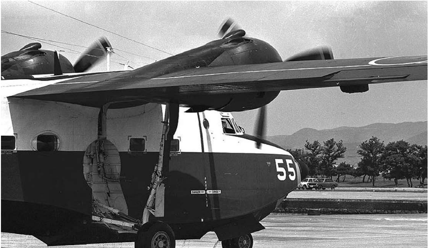
A Japanese UF-2 with the R-1820-82 engine. Note the different contour of the nacelle aft of the cowling. This is the same as the Canadian CSR-110.
