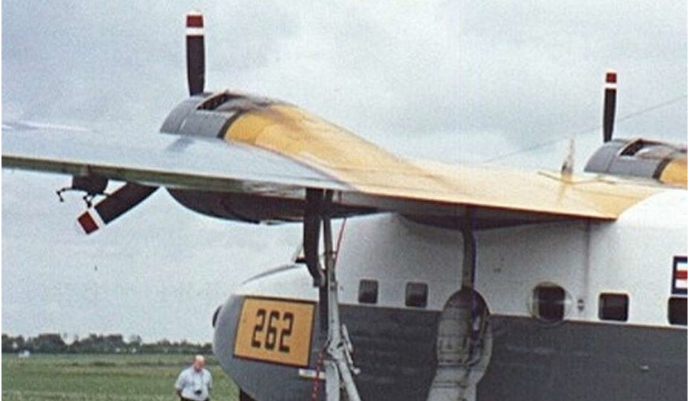
Seen from this angle you can make out the subtle bulges on the nacelle aft of the cowling. US Navy aircraft with R-1820-76 in the original configuration nacelle.
