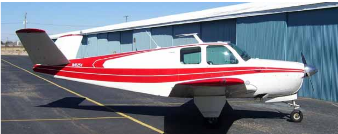
An original version Beechcraft 35. Note the two cabin windows and narrower tailplane...
