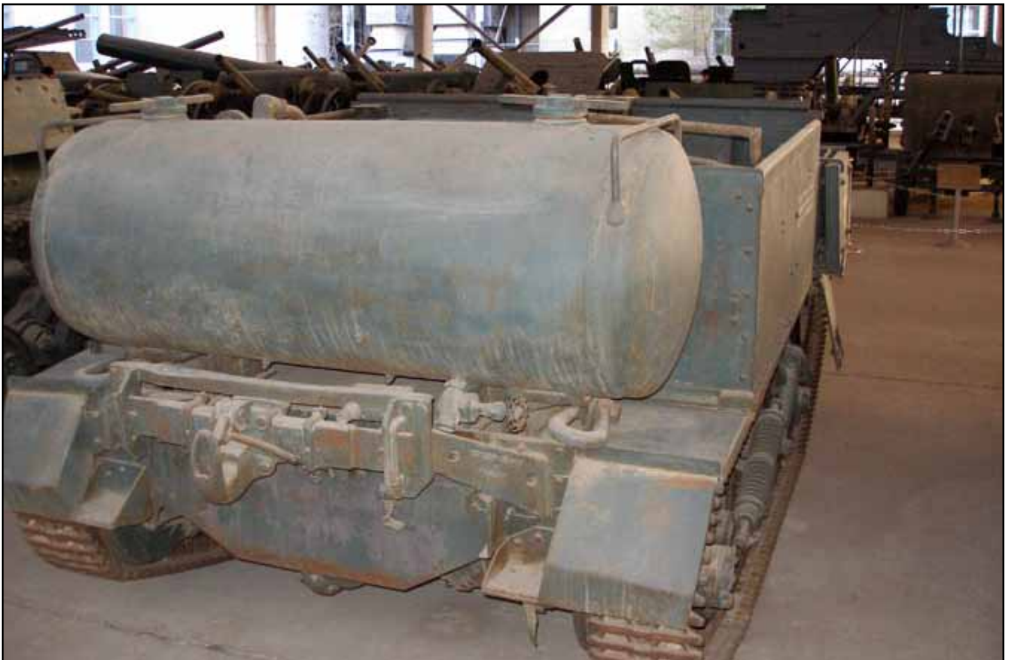
Externally mounted fuel tank and towing hook detail.
