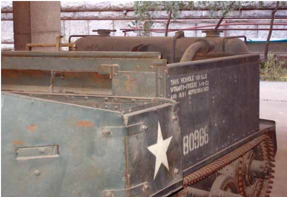
Air intakes and fuel pipe feeding from the rear tank.
