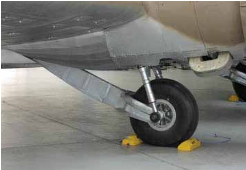
An Anson Mk I. Note the yoke-style single radius rod undercarriage (here covered with a fairing). That 'thing' in front of the undercarriage projecting from the nacelle is the oil cooler.
