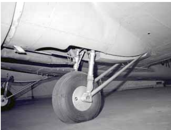
Undercarriage on the Anson Mk. V, similar to that of the Mk. II.
