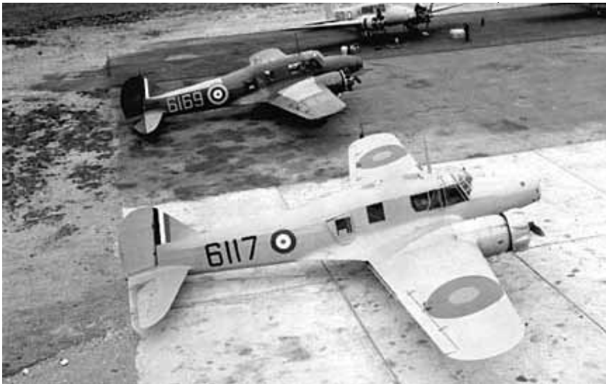
Anson Mk. Is, 6117 and 6169, in two different colour schemes. Arriving from the UK in camouflage finish, they were probably painted overall yellow as they underwent repair or overhaul. The fact that 6117 has had several cabin windows blanked off seems to reinforce that it has indeed been modified. The combination of dull type B wing roundels and what appear to be bright fuselage roundels is also interesting.
