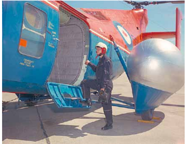
Some very nice modelling detail of RCAF H-44A 9591 in 1968, which was similar to the H-21A/B. Note the silver-fabric sea flotation bags fitted on this aircraft. (DND Photos PCN68-429 and PCN68-430)
