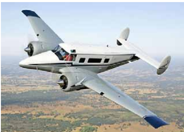
A Beech Super 18 (not Redding's aircraft). Note the long pointed nose and extended wingtips.
