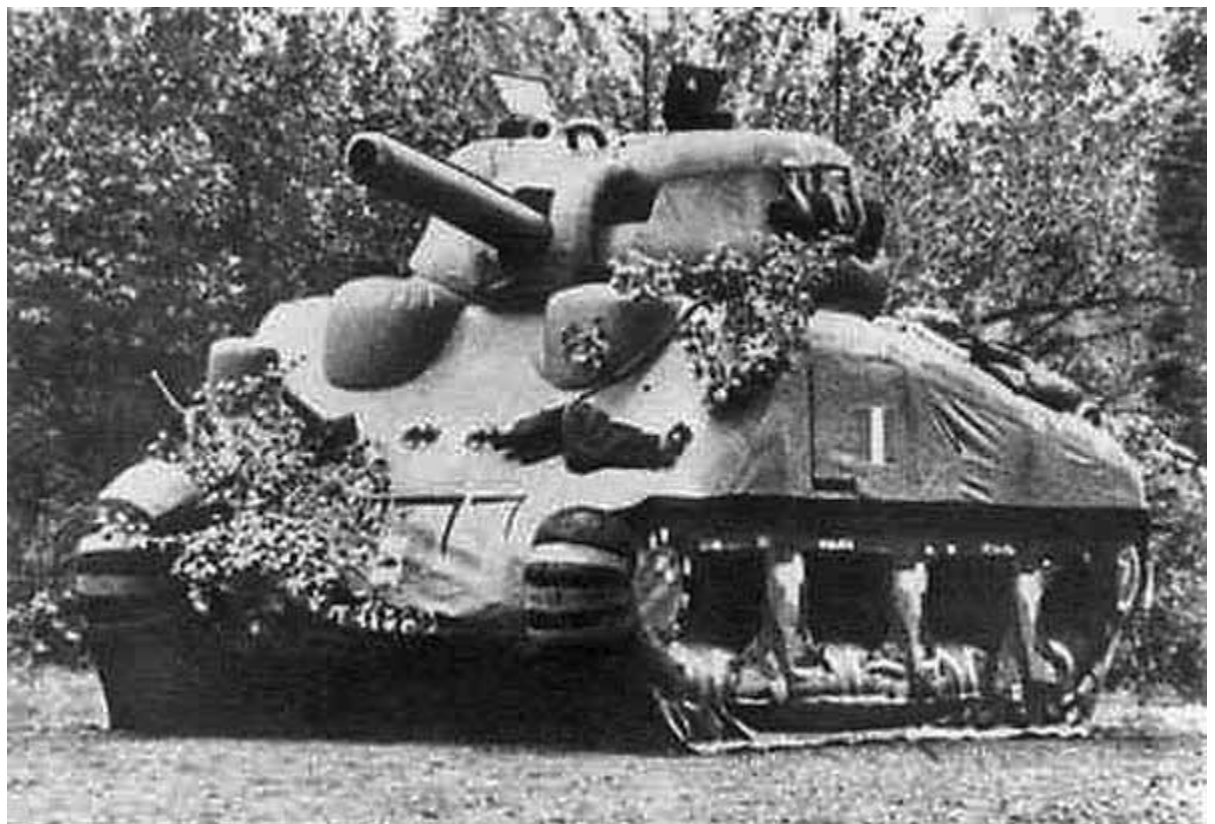
This Sherman is very realistic for an inflatable dummy. Note the open turret hatch and addition of some camouflage and gear on the hull.
