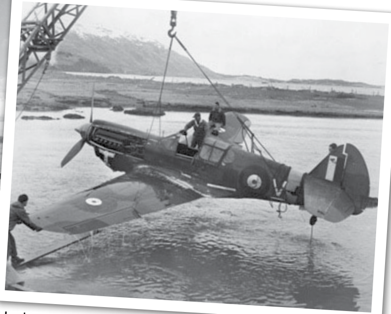
Having gone off the runway, AL194, aircraft "V" is hoisted from the water. Note that the red centre of the type B wing roundel has been over-painted with white, except for a tiny red dot. The Thunderbird emblem is carried on the nose.
