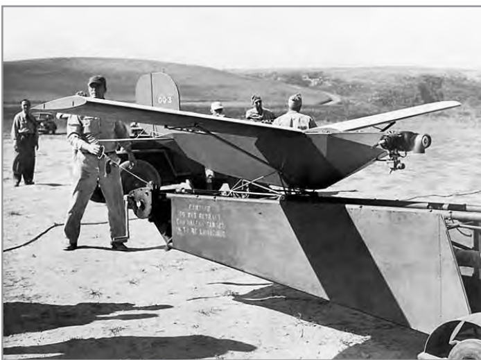
Above: An OQ-3 drone, its engine running, about to be launched. Right: Another OQ-3, on a somewhat more sophisticated launch ramp.
