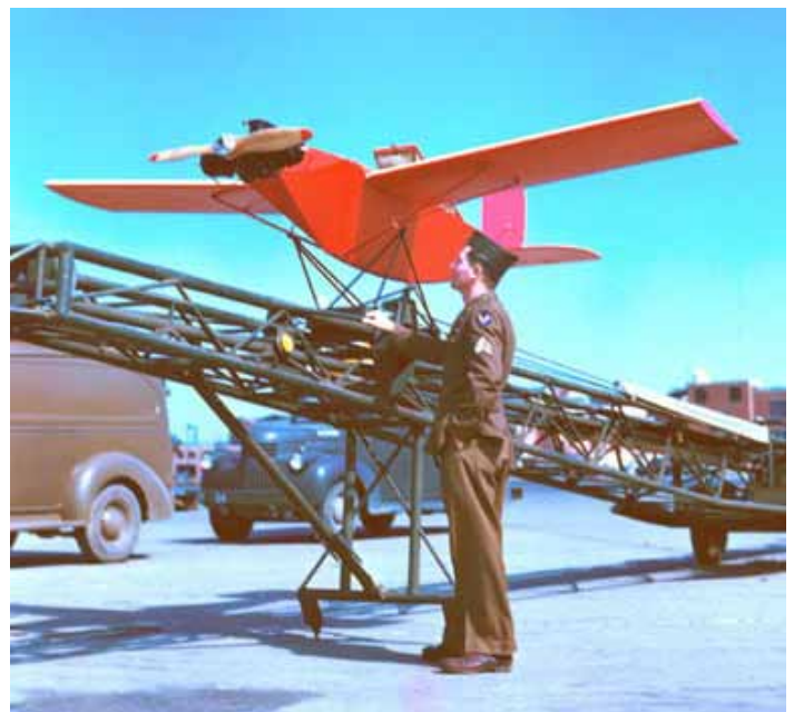
Above: An OQ-3 drone, its engine running, about to be launched. Right: Another OQ-3, on a somewhat more sophisticated launch ramp.
