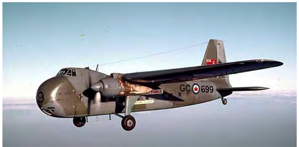
GC-699 in three-colour 1 Cdn Air Div camouflage. Note how the nacelle discolours aft of the exhaust.
