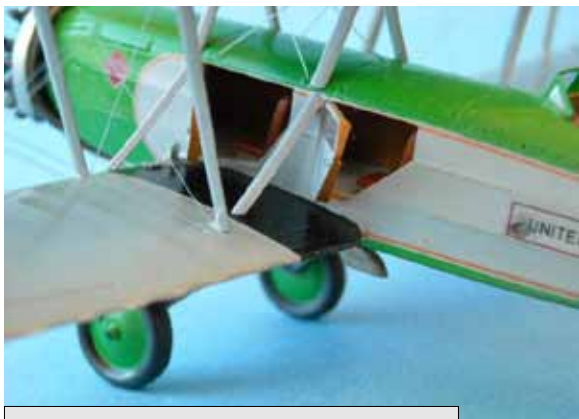
Showing the open doors. They are supplied in clear resin. I clued plastic sheet on the bottom and framing around the windows to the door some depth as shown on pictures of the real aircraft.
