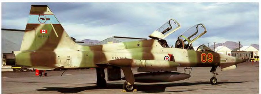
CF-5D 116809 in its Lizard scheme wraparound camouflage colours of FS30118 (brown), FS33531 (beige), and FS34258 (green). At this point it now carries the 419 Sqn tail band and 'slime' lights.
