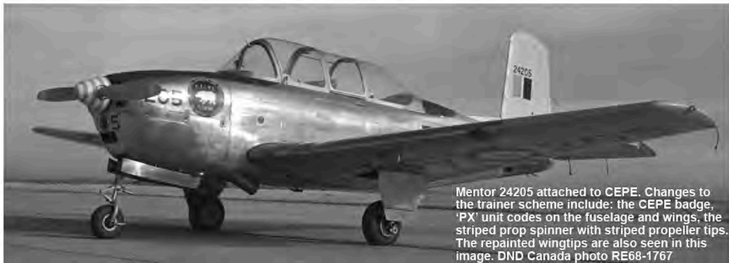
Mentor 24205 in regular RCAF service, carrying the trainer scheme of the day. The fin, rudder, tailplanes, elevators, wing tip caps and ailerons were 1-GP-12b Yellow 5-2.
