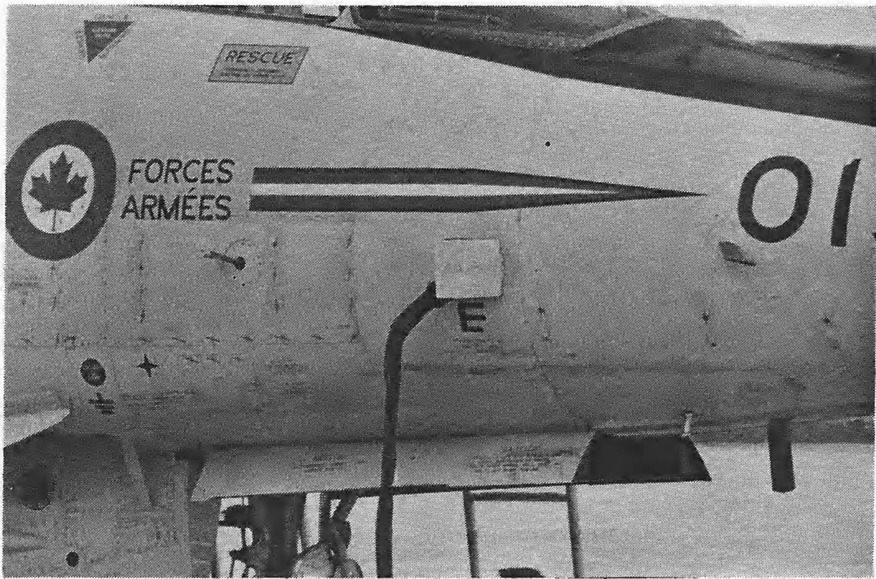
The angle of attack sensor, visible below the lettering "FORCES ARMÉES", is common to interceptors of both early and later series. Just behind and beside the UHF antenna under the nose is the temperature probe.
