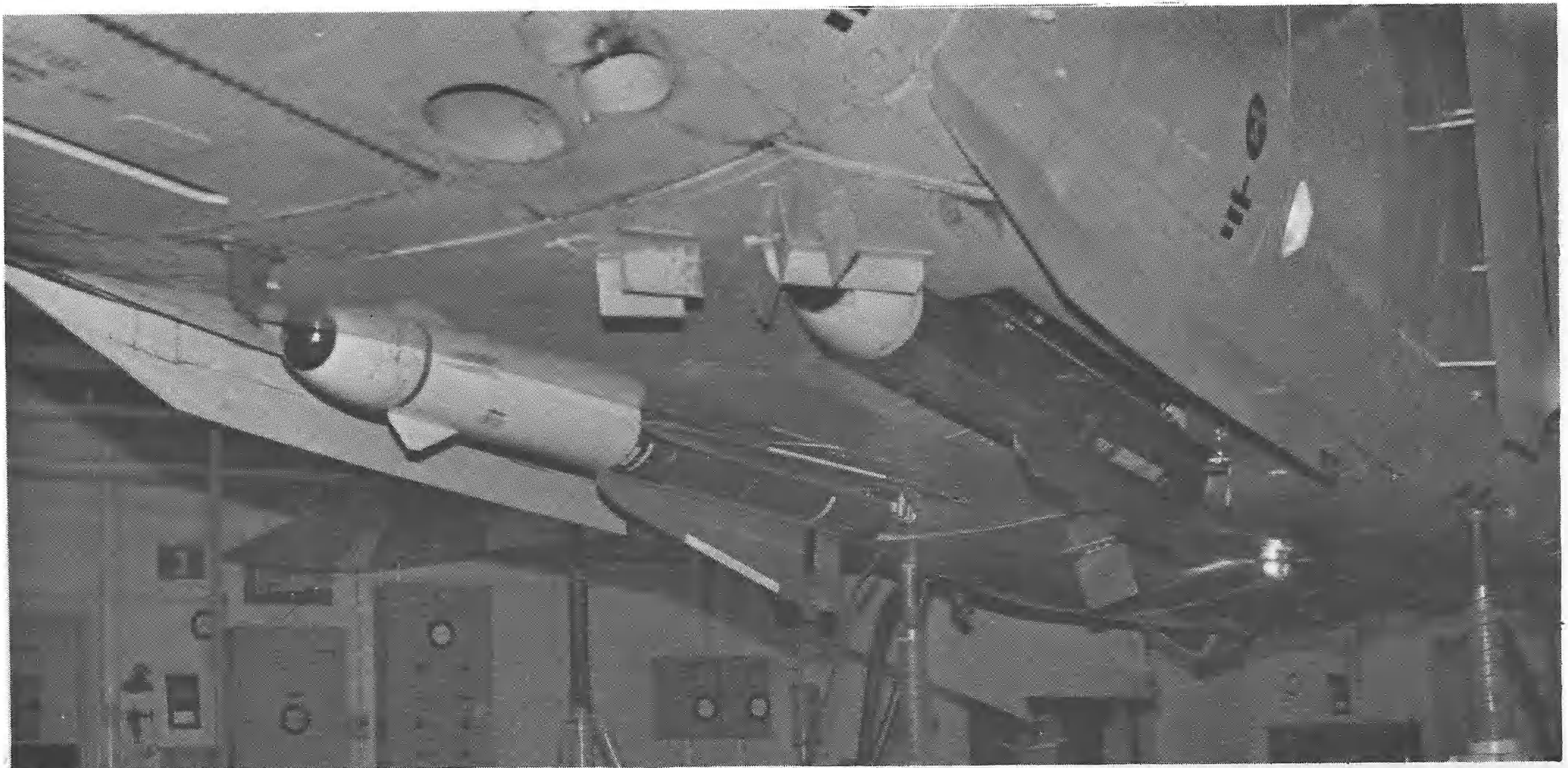
Above, an AIM-4D Falcon and a WSEM installed in their semi-flush mounting on the other side of rotating weapons bay door. Note the series of baffles and deflection plates in front of the port side WSEM. (Editor's Note: As a guess, I'd say the plates are meant to protect the sensing head of the port side Falcon when the first missile is fired from the starboard side. Anybody know for sure?) Below, two missiles deployed for firing. Note nosedown attitude. Rails are black. Also, note the slot visible when nosewheel doors are closed.
