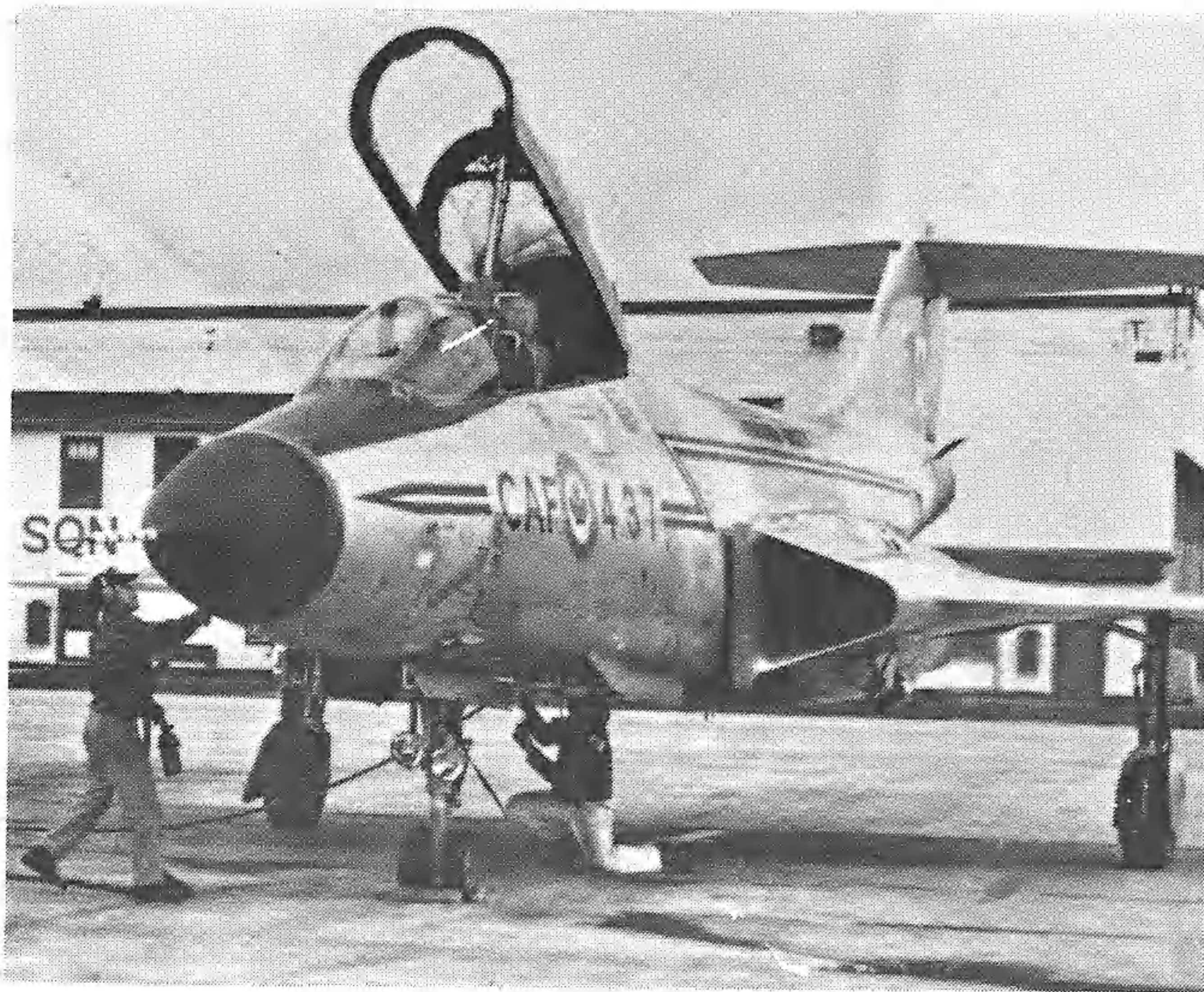
Above left, a first series CF101. Above right, a second series Voodoo. The first series had a protruding intake scoop for cooling equipment on the lower port nose beside the nose wheel well. The second series had a flush NACA type inlet in the same position. Look closely! Other differences are that the first series had a radio compass sense antenna, angle of attack transmitters rather than alpha probes and no IR sensor. On the photo at right, you will notice two vanes in the engine air inlet. These are only on second series 'F' models and were fitted in an attempt to improve airflow. Below, a better view of the single vane 'B' model inlet.
