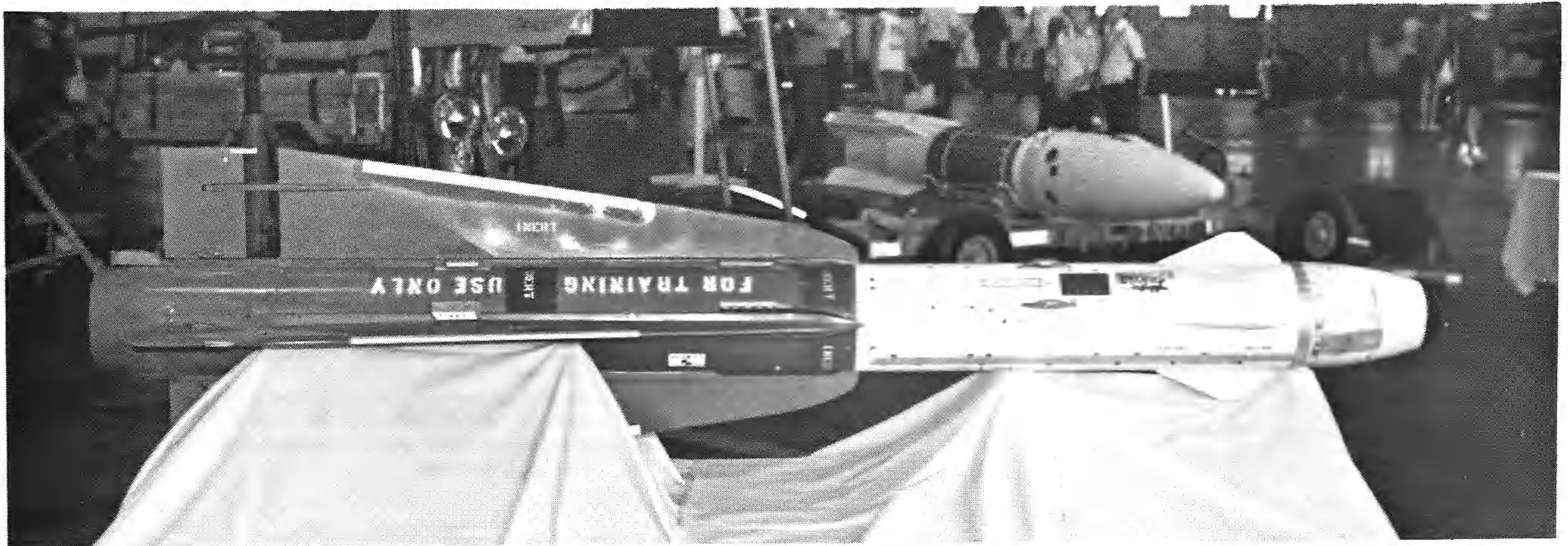
Above, the AIR-2A Genie rocket. Actually this is an ATR-2N used to train personnel on loading procedures and is gloss white with a dark blue band. On the real Genie, the tail fins extend in flight to stabilize the weapon. Here you might be able to see crossed wire tail bracing used on inert examples. Below, an AIM-4D Falcon. Forward section white, rear red. The thin bands on the leading edges of the fins are the detonators.
