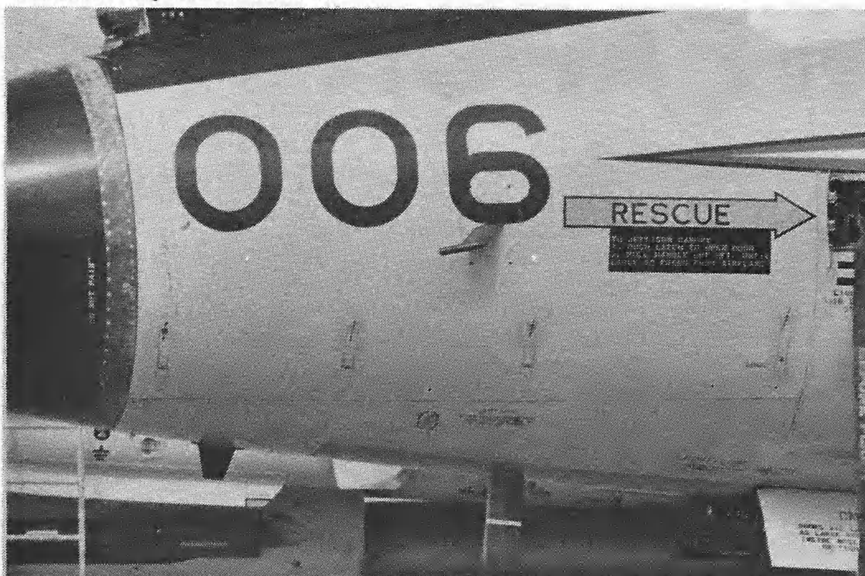
Below the alpha probe is the UHF antenna, metallic with a white stripe. Ahead we can see the black TACAN blade antenna, installed behind the radome only on CF101F's.
