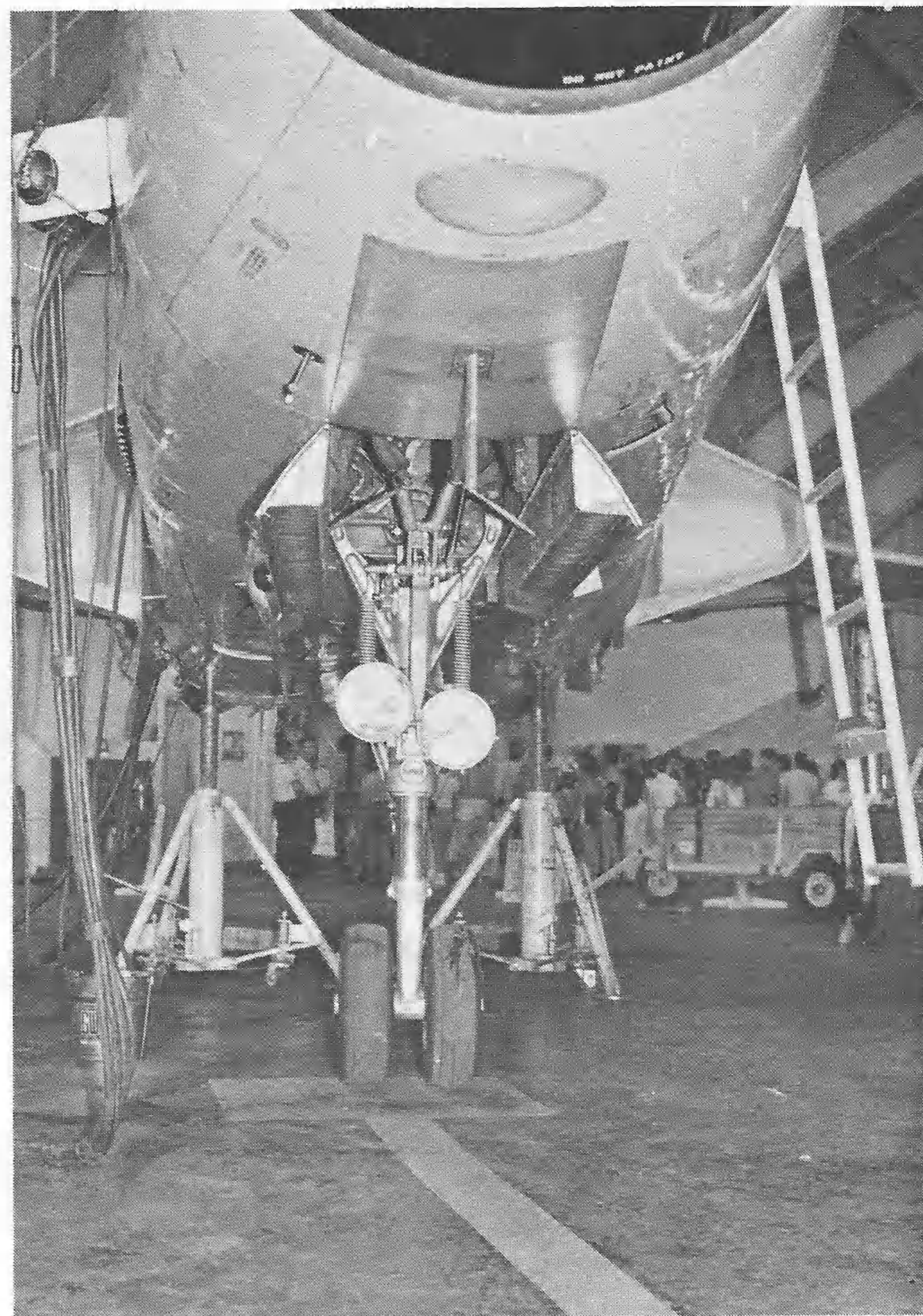
Front view of the nose gear. Note again the landing lights. The rectangular and round dielectric panels ahead of the wheel well are grey-green fiberglass.
