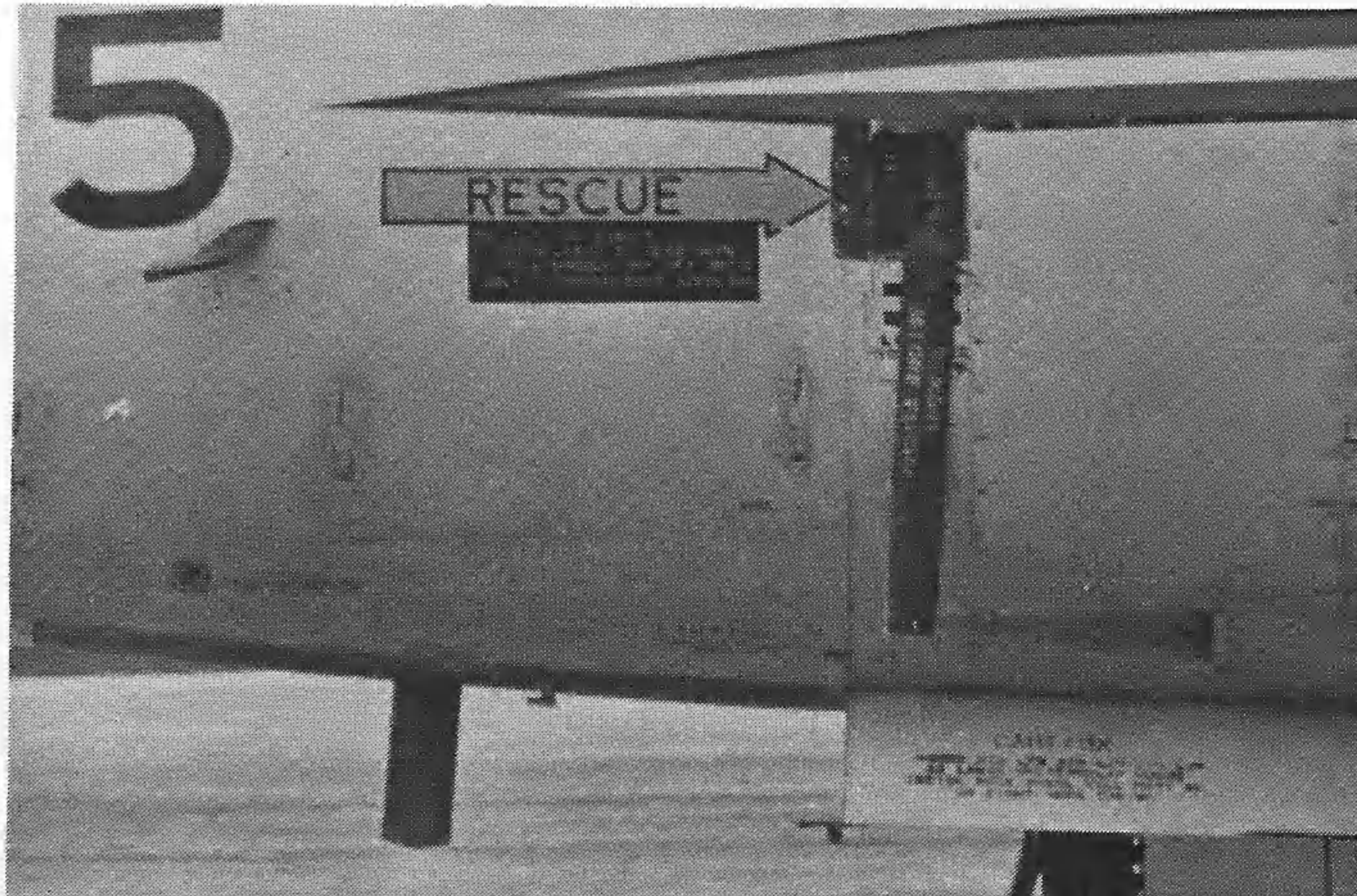
Second series a/c like this are equipped with an alpha probe on each side of the nose which furnishes data to the computer of the autopilot. On the first series, there were AOA sensors located here, in addition to the one highlighted above left.
