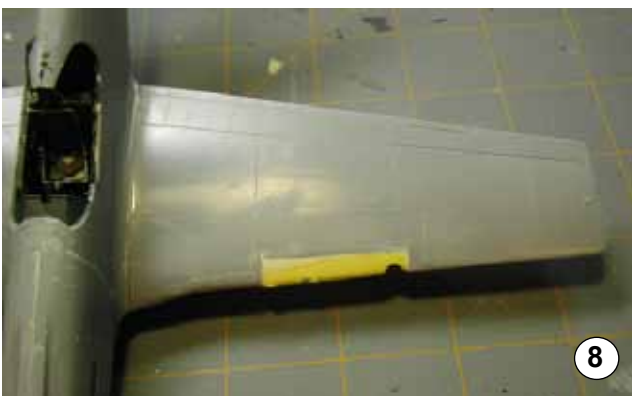
8 The wing insert on the port wing. The amount of filler is an indication of the not-so-precise cuts made.
