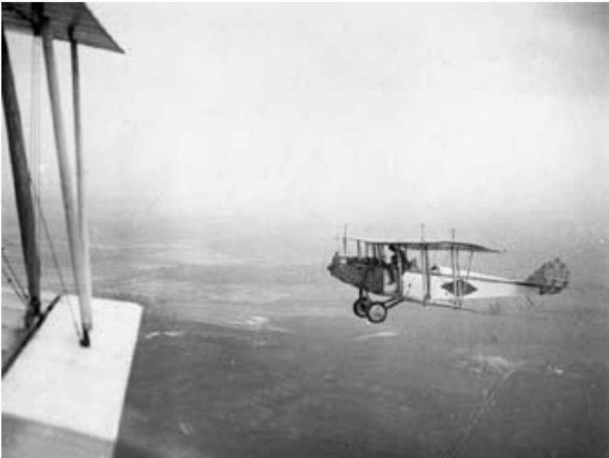
Two photos showing the V-shaped aileron struts to advantage. On the left, in flight somewhere over Central Ontario, and on the right a museum display.
