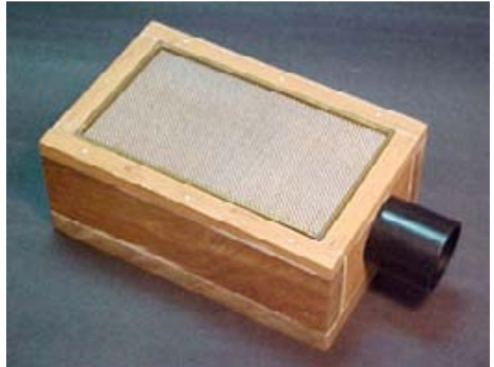
A similar vacu-former built sturdily of wood. There is no weatherstripping (yet) on this box.
