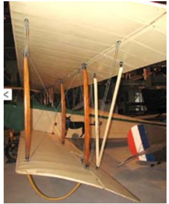
Two photos showing the V-shaped aileron struts to advantage. On the left, in flight somewhere over Central Ontario, and on the right a museum display.
