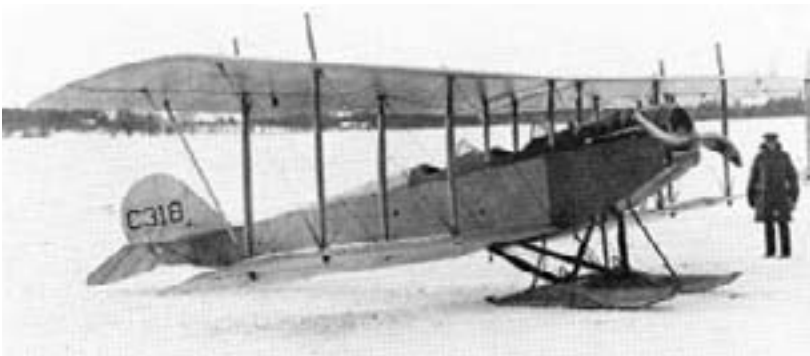
JN-4 Canuck #C318 fitted with skis for operation on snow covered airfields.
